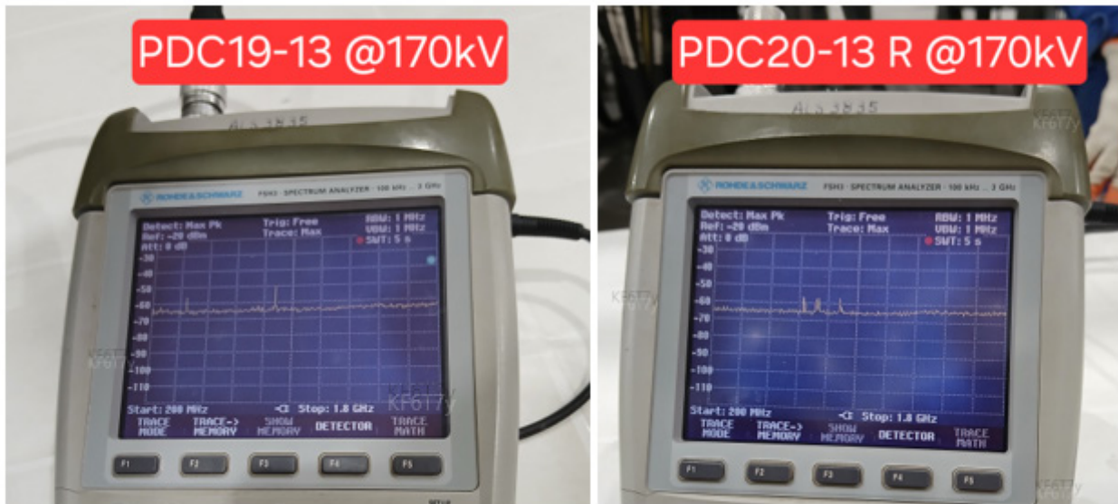
Figure 34: PDC20/19R - 13 After cleaning the gas compartment
