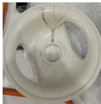
The Insulating cone located on gas section G22 had surface discharge and was failing Hipot test, tripping at 300kV
