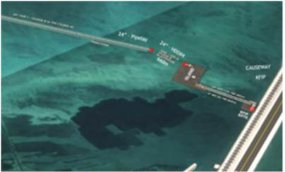
HDD#5 and HDD#6 were drilled from the third artificial island, KFIP Extension, towards Island A. The pipe strings were pre-welded on Island A and placed on carrying rollers for entire length. As all pipelines are internally protected by CLAD liner, the weld was made from a stationary welding area and pulled until HDD entry location by a linear winch, in preparation for final HDD pullback. The HDD crossing was made under the KFIP access causeway.
